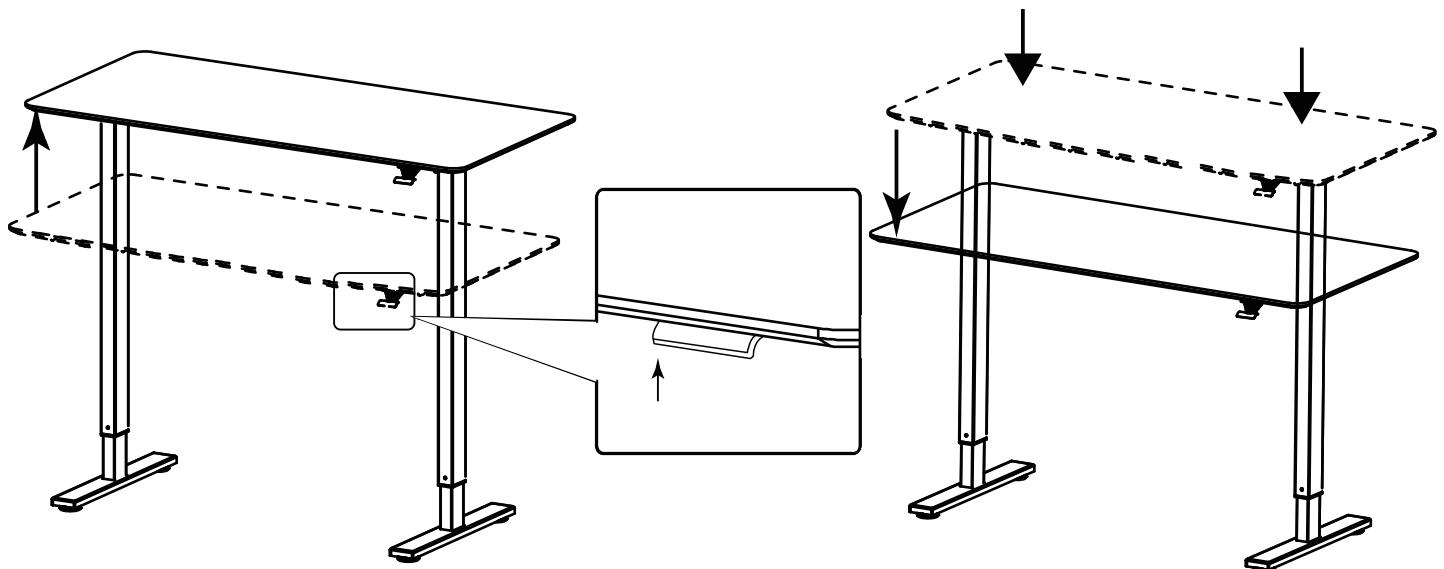
Lift the paddle for lifting the table top.
